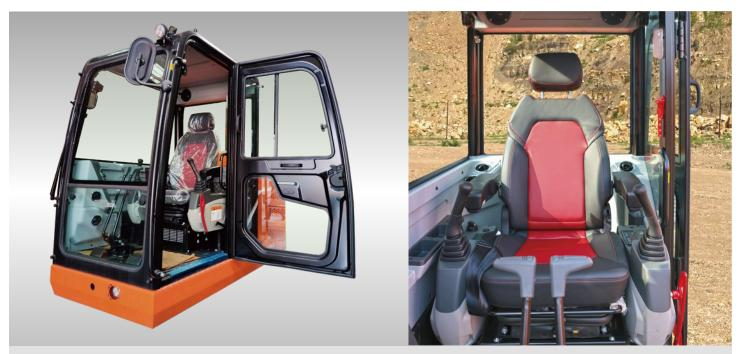
Equipped with suspended leather seat and ergonomically optimized pilot control system to alleviate operating fatigue effectively
