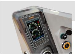
Equipped with one-button start and **5.7 inches LCD**, man-machine interaction is more convenient and intelligent.
